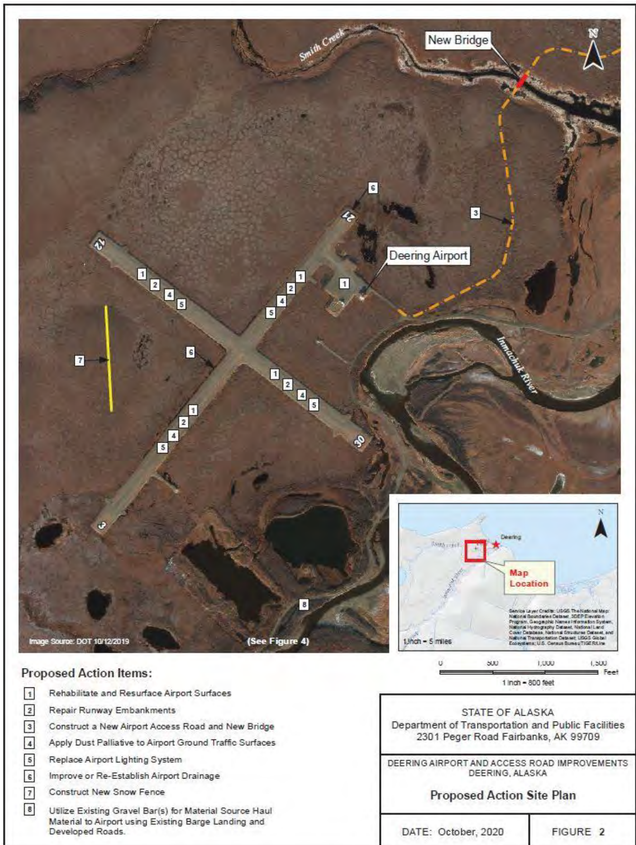
Figure 2. Detail of the proposed airport and access road improvements, including the new Smith Creek bridge near Deering, Alaska.
