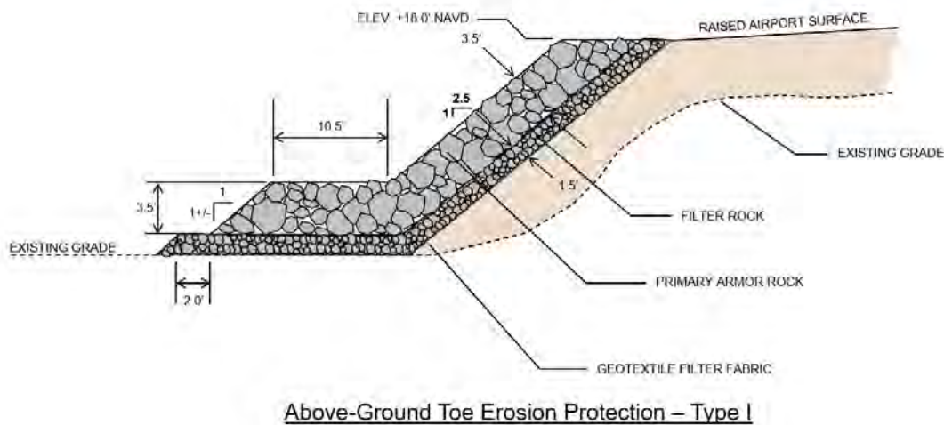
Figure 22: Example of an Above-Ground Toe Erosion Typical Section (Type I 2.5H:1V Concept Shown)
