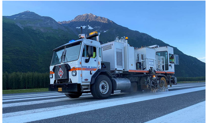
Tazlina District, Ernestine crew painting Valdez Airport. Photo by Chance Box, Alaska DOT&PF
